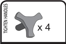
Always secure all four adjustment handles before cycling. Make sure that the handlebar is not slided beyond its outermost position.
