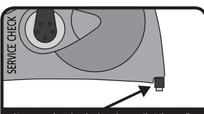
At an annual service check, make sure that the small hole by the front bottom frame is not blocked and allows water and sweat to exit the frame. Also check that the ribs on the poly-v belt and pulley are clean.
