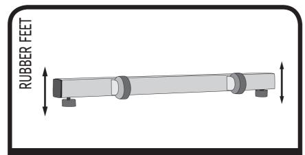
The rubber feet should always be adjusted to ensure that the cycle is in level. Every other year the rubber feet should be replaced as the rubber hardens and becomes unable to absorb the impact.
