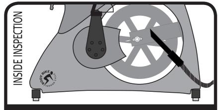
Inspect the Kevlar brake pad after the first month and hereafter every 3rd month. The Kevlar brake pad should be replaced before it is worn through and reveal the black rubber. At every inspection the bike should be vacuum cleaned inside.
