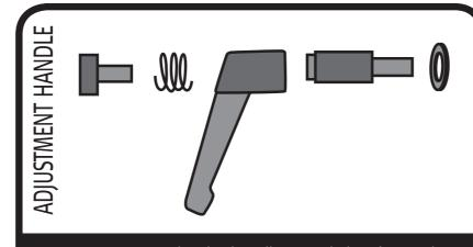
Every 3 months the handles need cleaning and grease. Disassemble the handle completely. Clean all the parts thoroughly using a steel brush. Lubricate the internal parts with grease. Add grease to the main screw before mounting it on the cycle.
