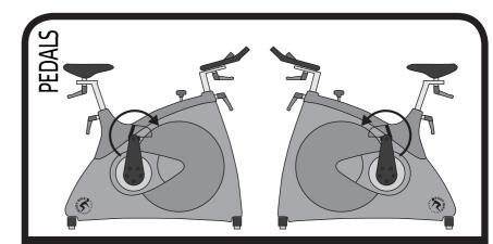
Tighten up the pedals every 2 weeks to avoid them getting loose or breaking off. The pedals should always be screwed on in the direction of the handlebar. Use a 15mm pedal wrench to tighten the pedal. Pedals should be changed once a year or after 1500 hours of cycling.
