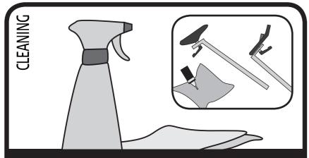
After each workout, wipe the cycle down with tissue paper. Every other week the posts need cleaning to protect them from sweat etc. Pull out the seat post and the front post and wipe them clean with an oily cloth.
